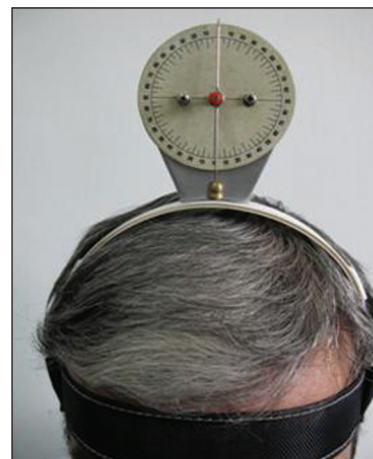
Figure 2: Status of tiltometer over the patients head during autorefractometry
